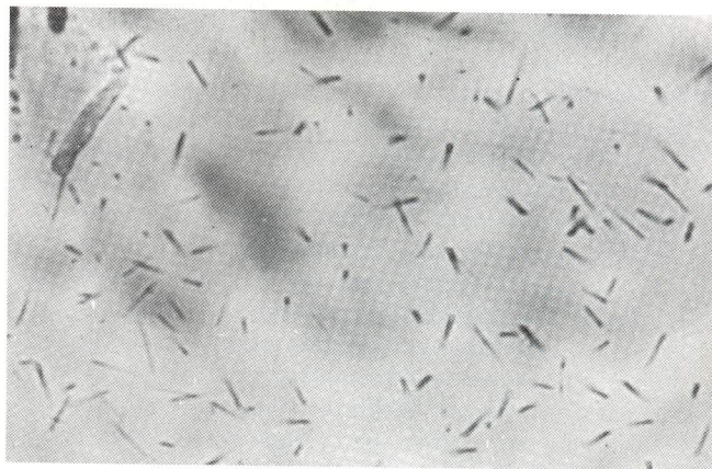
FIGURE 9-26 Each fission track (about 16 \mu in length) in this apatite crystal is the result of the radioactive decay of a uranium atom. In order to make the fission tracks visible, the apatite crystal has been etched with hydrofluoric acid. This apatite crystal comes from one of the dikes of Shiprock, New Mexico, and indicates a calculated age of 27 million years. (Photo courtesy of Charles W. Naeser, U.S. Geological Survey.)
